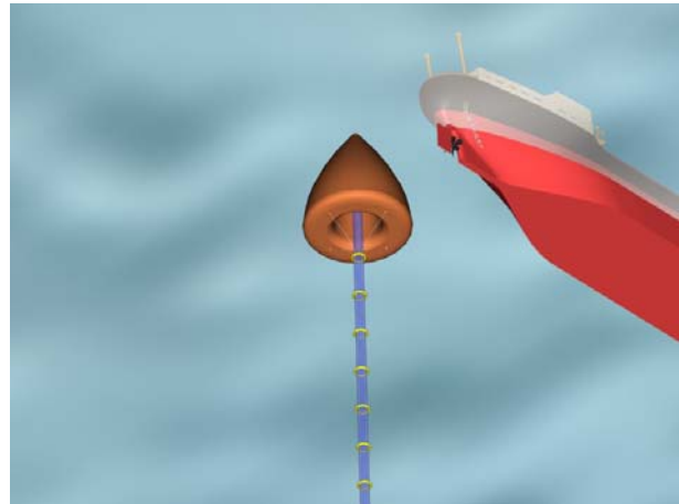
Fig. 6: Riser Tube, Buffer Bell and Shuttle tanker
